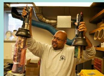
A BGC float sensor head on the left, and a Core Argo one on the right
