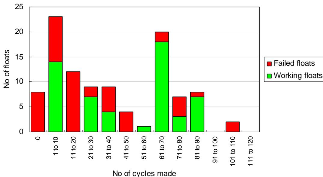
Showing the performance of UK floats deployed (excluding 2 floats which were not correctly deployed) as at early February 2004.
