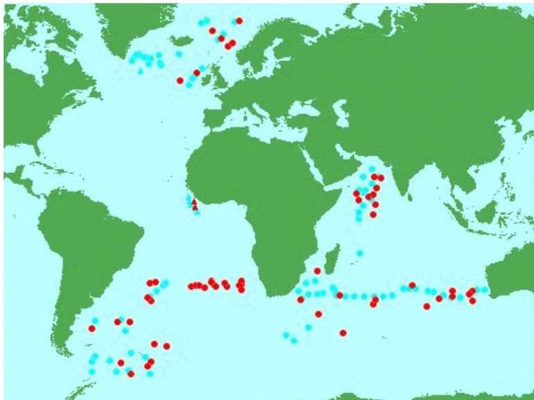
*Showing locations at which UK floats have been deployed ● and current positions ● of those reporting (February 2004). Circles show Apex floats, triangles Provor floats. Figure includes the Mauritius float and 2 Irish floats (deployed in the Rockall Trough) being processed by UK Argo.*
